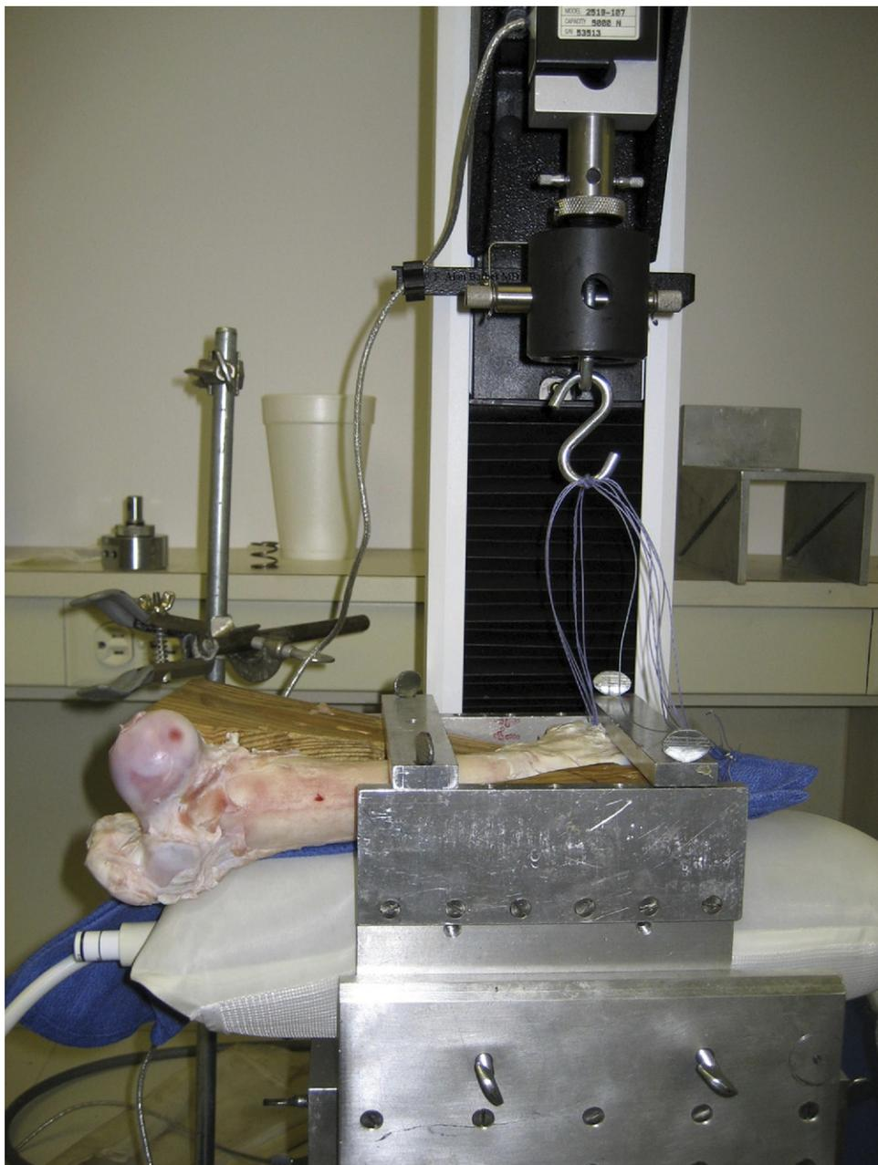
**FIGURE 5.** Mechanical testing machine setup used for anchor testing. © 2011 F. Alan Barber.
